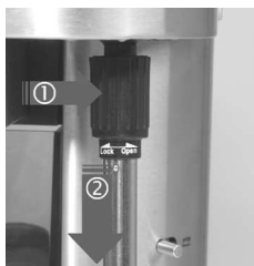
① Touch the stainless steel nozzle at its shaft for removing, turn it to the right and unlock it. ② Then, pull the stainless steel nozzle down.
