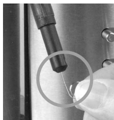
Clean the outlet hole of the hot water/steam nozzle thoroughly!
