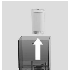
Step 2: Remove filter cartridge.
