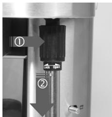
① Touch the bush at its shaft for removing, turn it to the right and unlock it.
