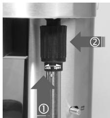
① Touch the stainless steel nozzle at the shaft for attaching it and push the nozzle on.
