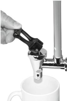
Turn the tap-handle until its half-round underside faces to the front. To dispense liquid, tip the tap-handle to the front and keep it until the desired amount of liquid has been drawn off. To stop dispensing, just let the tap-handle go and it will return to its upright position and close the tap automatically.
