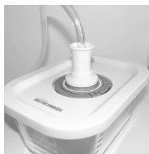
With the hose adapter, the VCG 1 containers can be used with all Rommelsbacher bar vacuum sealers. Connect the hose plug to the container connection of the vacuum sealer, press the suction connection lightly onto the container valve and then start the container function on the vacuum sealer. Many devices from other manufacturers have a compatible hose connection; the hose adapter can also be used here.
