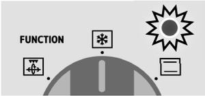
The appliance is equipped with a temperature pilot lamp. The pilot lamp expires once the set temperature is reached. The alternating lighting and expiring of the pilot lamp during operation indicates the thermostatic regulation of temperature.
