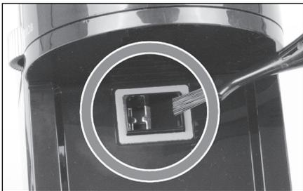
Remove sticking powder carefully by means of a pointed object (e. g. toothpick). Afterwards clean thoroughly by means of the enclosed cleaning brush.
