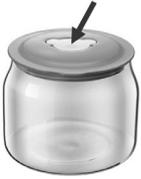
The lid of the glass container is equipped with a venting valve.
