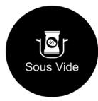
Sous Vide | <ul style="list-style-type: none"><li>• To select the <b><i>Sous Vide</i></b> direct selection programme, tap the corresponding touch key once. <b>60 °C</b> is selected as the suggested temperature.<br/>→ Tapping the touch key is confirmed with a signal tone and <b>60</b> appears in the left display field.<br/>→ The pilot lamp above the <b>ON/STANDBY</b> touch key is lit continuously.</li></ul> |
